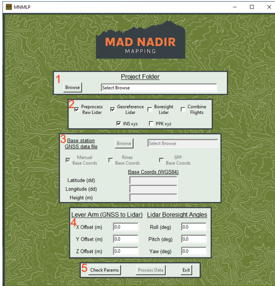
Figure 3: Main GUI window of the MNMLP software. The five individual GUI sections are labeled by red numbers
